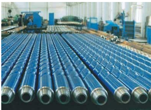
Figura 3.6: Drill Collars. (Fonte: http://www.chinaoilequipments.com/Drilling-Production/Drilling-tools/spiral-drill-collar.1099.htm )
