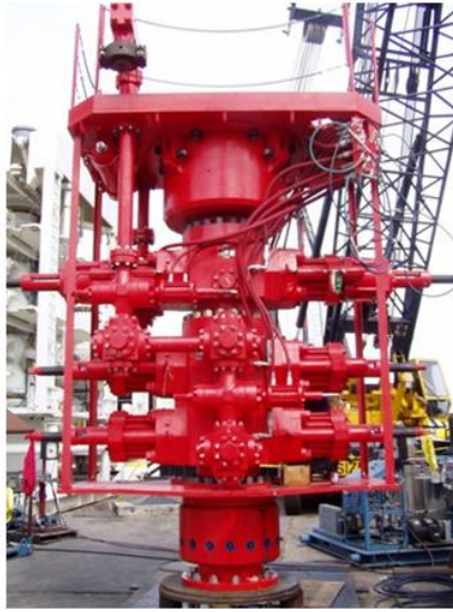
Figura 3.5: Blowout Preventor. (Fonte: http://www.shanglin-oilfield.com/pro_info.asp?id=41 )
